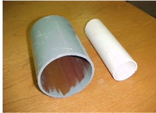
Biofilm contamination on chlorine-treated line (left) versus mixed-oxidant line (right) at Diana Water Supply
