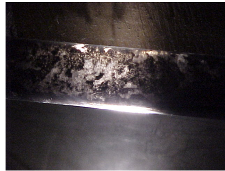
Breakdown of biofilm begins with mixed oxidants
